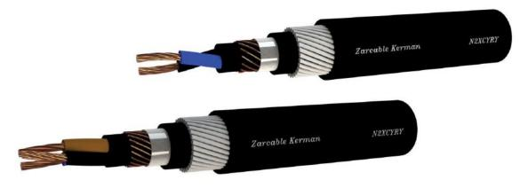
Armoured Power and signal cable 0,6/1 kV, XLPE insulated, PVC sheathed, with concentric protective Cu conductor
